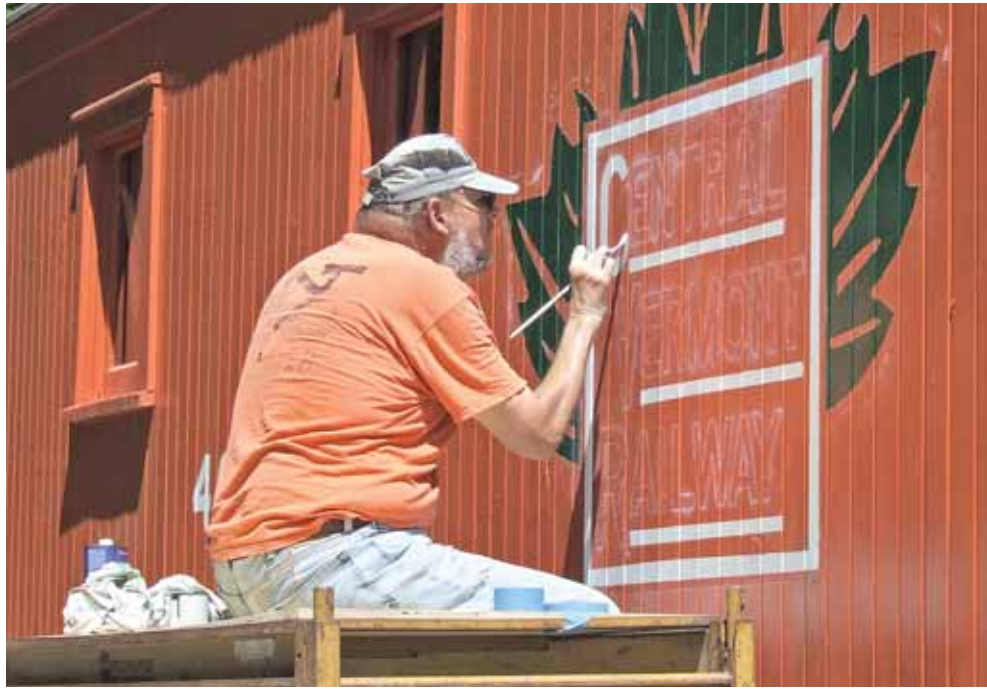
Al Pomeroy paints between the stencil lines to finish the maple leaf herald on the trail side of the caboose. Caption and photo: Bob Norander
